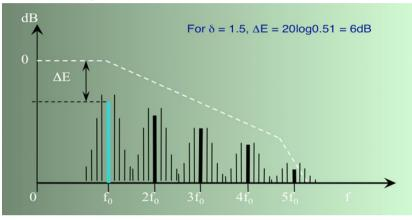
Figure 2 – Frequency Domain Representation of a Sinusoid Modulated Periodic Signal
